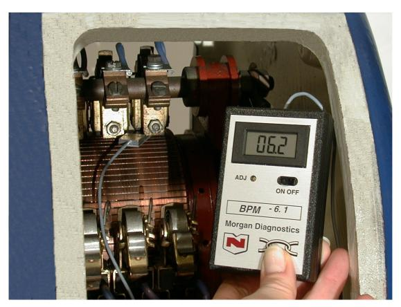
The large LCD display gives an immediate reading direct from the brush/commutator interface ranging from 0.1 to 50N - more than enough to check this critical parameter across the entire range of brushed equipment.
